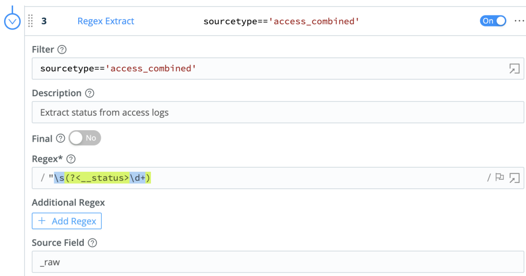
Extracting the __status field
